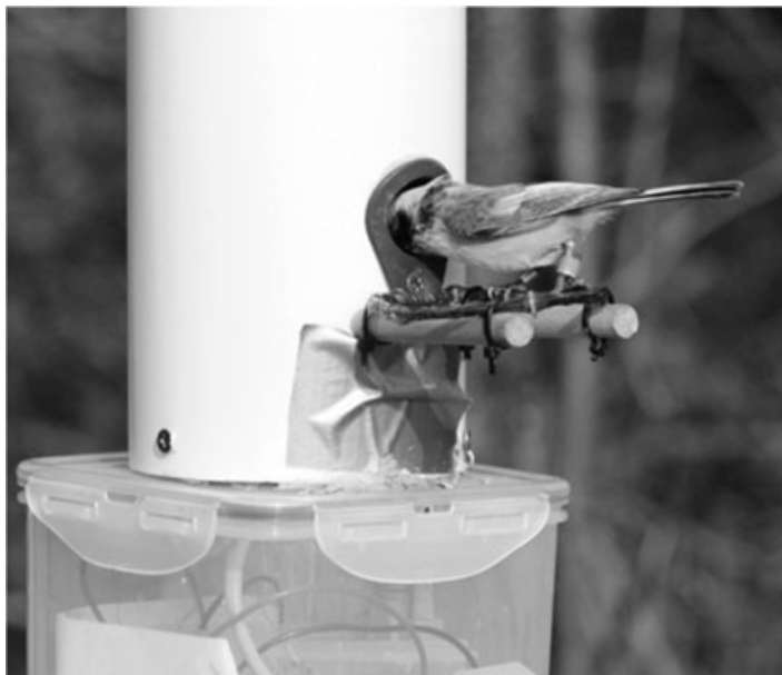
Fig. 2. Black-capped Chickadee with an RFID leg band using a feeder equipped with the low-cost RFID reader. The RFID antenna is located on top of two pieces of wooden dowel extending from the PVC feeder housing. The RFID reader and battery (not visible) are housed in a container attached to the bottom of the feeder. Photo, courtesy K. J. McGowan.
