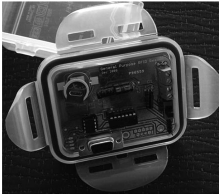
Fig. 1. Photo of completed circuit board mounted inside the lid of a waterproof 180-ml container (Lock N Lock, Blacktown NSW, Australia). Circuit board dimensions are approximately 80 mm × 60 mm.
